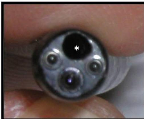
Figure 4: Trans-nasal Esophagoscope (TNE). The distal end of the scope has light, camera, and a working channel. The working channel port (*asterisk*) allows instrumentation to be passed to perform procedures.
