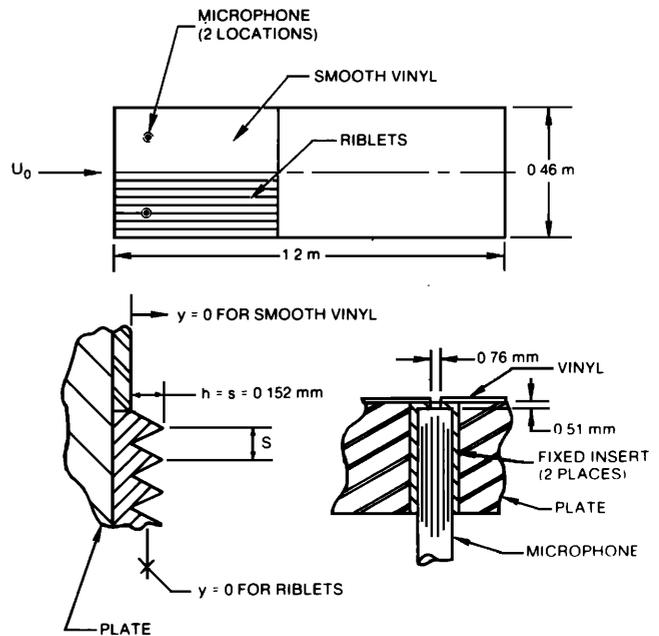
FIG. 1. Plate configuration.
