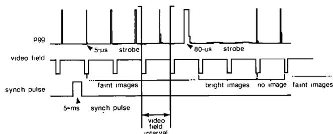
FIG. 2. Validation of timing of recorded images relative to strobe occurrence. Bright images were produced by the  $80\text{-}\mu\text{s}$  flash. Digitized waveforms: PGG recording of strobe, video fields, and synchronization pulse. Cursors depict the video field interval.
