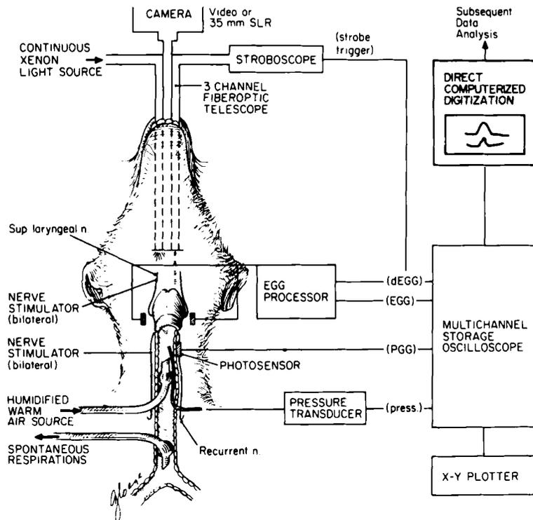
Fig 2. Schematic representation of experimental set-up for in vivo canine model of phonation. SLR — single lens reflex, EGG — electroglottography, dEGG — differentiated electroglottography, PGG — photoglottography.
