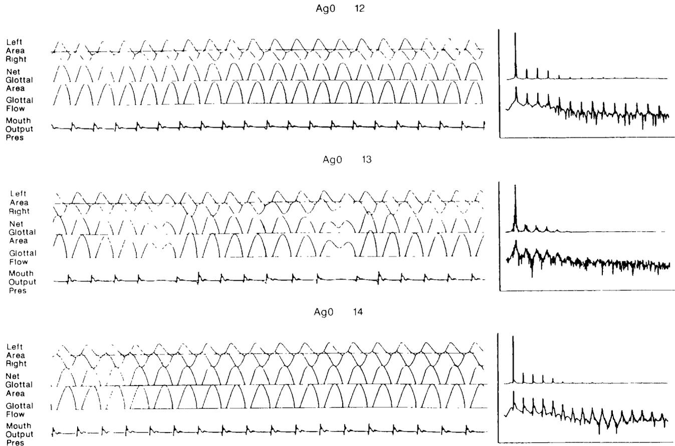
**FIGURE 5.** Time and frequency domain displays of recurrent paralysis simulations taken at  $A_{g0}$  of .12, .13, .14  $\text{cm}^2$ , corresponding to the region of speed quotient discontinuity ( $P_{sub} = 6 \text{ cm H}_2\text{O}$  side) in Figure 3.
