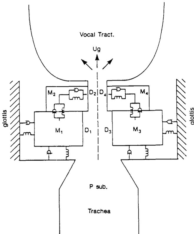
**FIGURE 1.** The four-mass model of larynx and vocal tract, after Koizumi et al. (1987, 1989). Note that each upper mass is coupled only to the lower mass, and not to the side wall (as is the lower mass). D = vertical distance; M = mass of each element;  $U_g$  = glottal flow;  $P_{sub}$  = subglottal pressure.
