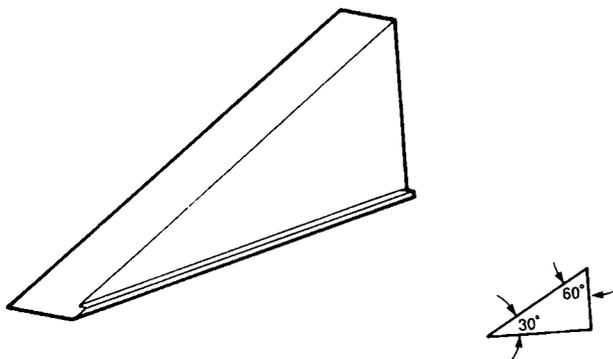
FIG. 2. View of the inferior surface of the triangle-shaped Silastic implant. The inset demonstrates the posterior angle ( $\sim 30^\circ$ ) and lateral angle ( $\sim 60^\circ$ ).
