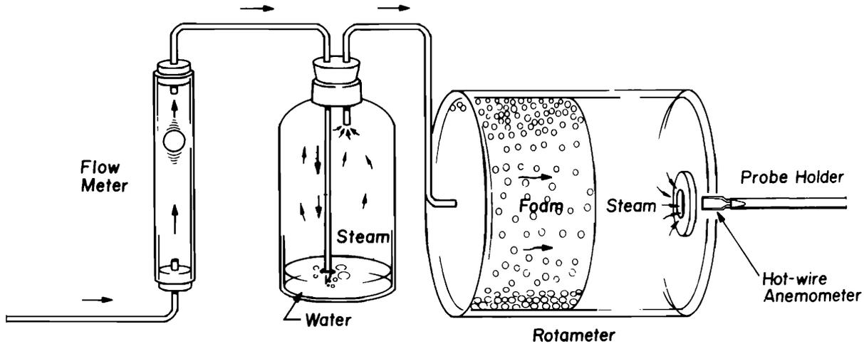
FIG. 2. Schematic of the constant-temperature anemometer calibration setup for air and helium with (1) Gilmont flow meter, (2) constant-temperature humidifier, (3) jet settling chamber with packing of open cell foam, (4) outflow jet, and (5) anemometer probe tip.
