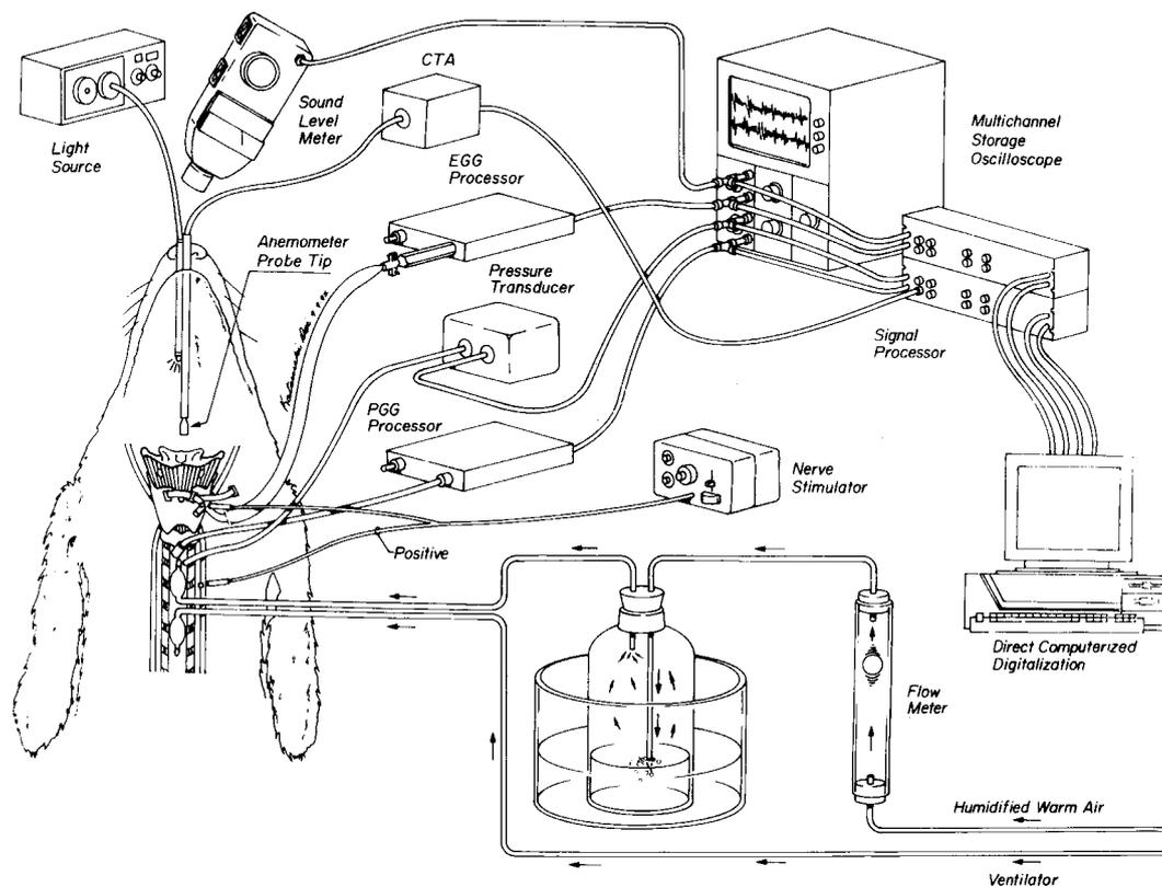
FIG. 1. In vivo canine model setup for collection of EGG, PGG, SGP, and anemometer data.
