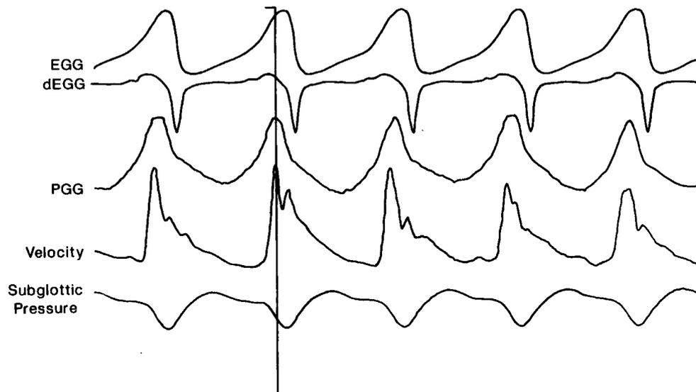
**FIG. 3.** Example of the simultaneous EGG, PGG, particle velocity, and SGP waveforms recorded in the experimental design. Note the doublepeaked velocity waveform.
