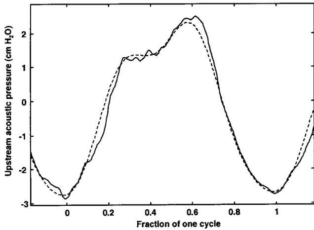
FIG. 9. Comparison between the measured upstream sound pressure and that predicted from the monopole source model and quasi-steady approximation.  $f=80$  Hz,  $\Delta p_0=12$ -cm  $H_2O$ , and convergent orifice geometry. —: measured; - -: predicted.
