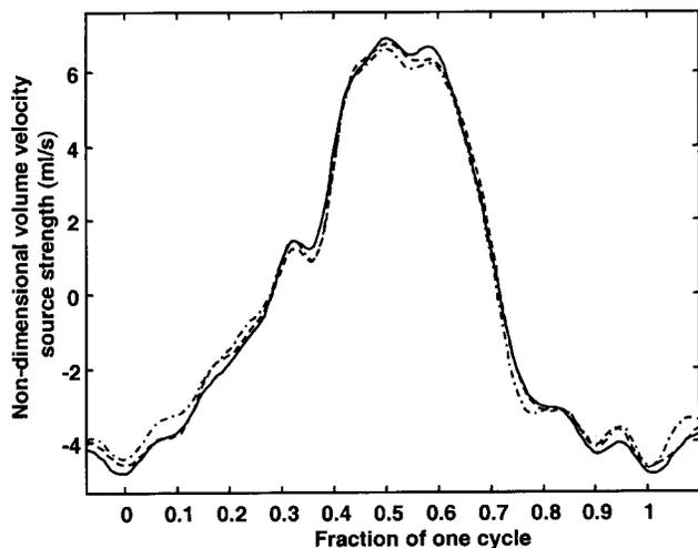
FIG. 12. Volume velocity source strengths at 120 Hz for three different mean pressure drops (6-, 9-, 12-cm H<sub>2</sub>O), and straight orifice geometry. The volume velocity source strength is scaled by the square root of the mean pressure drop. —: 12-cm H<sub>2</sub>O; - - : 9-cm H<sub>2</sub>O; ···: 6-cm H<sub>2</sub>O.
