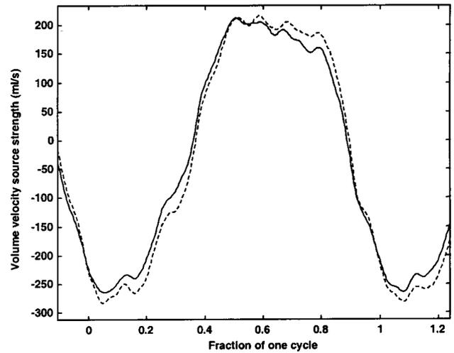
FIG. 8. Volume velocity source strength at the origin calculated based on the measured sound pressure and the reflection coefficient measured simultaneously at the same experiments.  $f=80$  Hz,  $\Delta p_0=12$ -cm  $H_2O$ , and convergent orifice geometry. —: upstream; - -: downstream  $\times(-1)$ .
