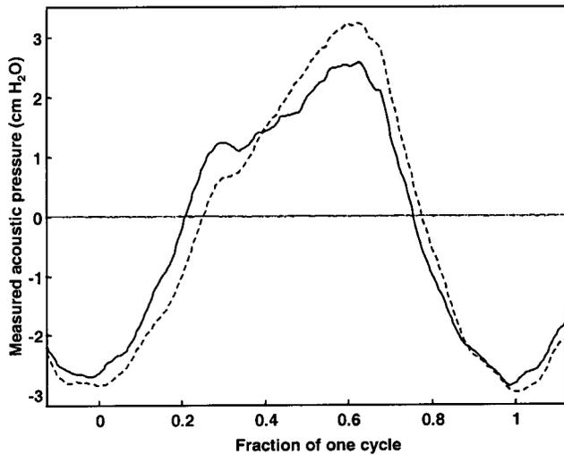
FIG. 7. The measured upstream and downstream unsteady pressure in the convergent orifice case.  $f=80$  Hz,  $\Delta p_0=12$ -cm  $H_2O$ . —: upstream; —: downstream  $\times(-1)$ ; - -: upstream background noise; - -: downstream background noise.
