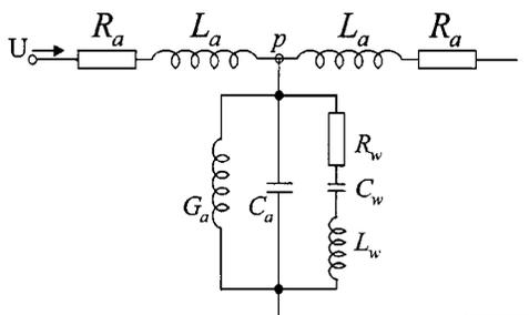
FIG. 4. Transmission line representation of the vocal tract.
