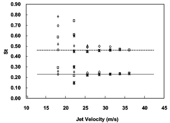
FIG. 14. The Strouhal number of the observed jet tones for a divergent glottis-shaped orifice versus the jet velocity. □, confined air jet; △, confined CO<sub>2</sub> jet; ◇, confined He-CO<sub>2</sub> jet; \*, free air jet; +, free CO<sub>2</sub> jet; —,  $St = 0.23$ ; - - -,  $St = 0.46$ .
