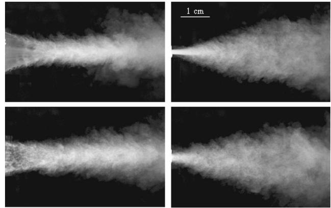
FIG. 17. Flow visualization of free jet just beyond the convergent (top) and divergent (bottom) orifices.  $\Delta p = 4$  cm H<sub>2</sub>O. The jet in the first 5 to 10 mm is clearly more stable in the convergent case than for the divergent case.
