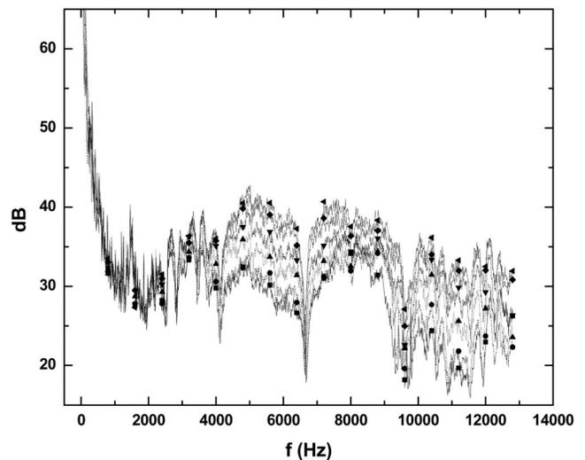
FIG. 12. Sound spectra measured at different high flow rate in air. Free jet flow through a divergent glottis-shaped orifice. ■,  $\Delta p = 10$  cm H<sub>2</sub>O; ●,  $\Delta p = 12$  cm H<sub>2</sub>O; ▲,  $\Delta p = 16$  cm H<sub>2</sub>O; ▼,  $\Delta p = 20$  cm H<sub>2</sub>O; ◆,  $\Delta p = 26$  cm H<sub>2</sub>O; ◀,  $\Delta p = 30$  cm H<sub>2</sub>O.
