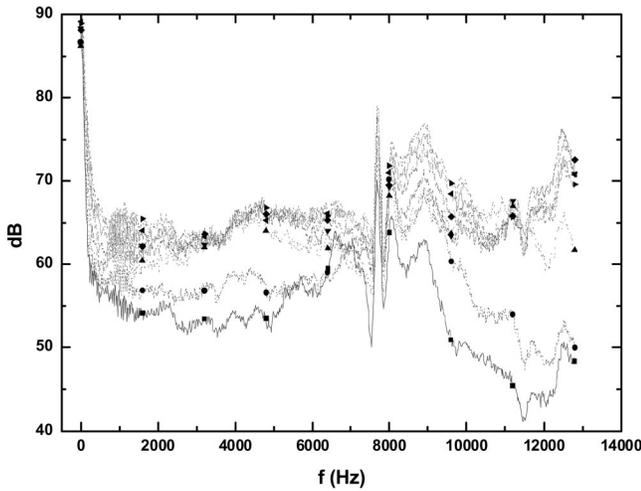
FIG. 9. Sound spectra measured at high flow rate in air. Divergent glottis-shaped orifice. ■,  $\Delta p = 9$  cm H<sub>2</sub>O; ●,  $\Delta p = 10$  cm H<sub>2</sub>O; ▲,  $\Delta p = 14$  cm H<sub>2</sub>O; ▼,  $\Delta p = 18$  cm H<sub>2</sub>O; ◆,  $\Delta p = 22$  cm H<sub>2</sub>O; ◀,  $\Delta p = 26$  cm H<sub>2</sub>O; ▶,  $\Delta p = 30$  cm H<sub>2</sub>O.
