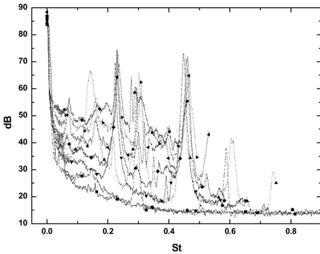
FIG. 13. Sound spectra measured at low transglottal pressures in air. Divergent glottis-shaped orifice. Pure tones were observed. ■,  $\Delta p = 1$  cm H<sub>2</sub>O; ●,  $\Delta p = 2$  cm H<sub>2</sub>O; ▲,  $\Delta p = 3$  cm H<sub>2</sub>O; ▼,  $\Delta p = 4$  cm H<sub>2</sub>O; ◆,  $\Delta p = 5$  cm H<sub>2</sub>O; ◀,  $\Delta p = 6$  cm H<sub>2</sub>O; ▶,  $\Delta p = 7$  cm H<sub>2</sub>O; ●,  $\Delta p = 8$  cm H<sub>2</sub>O.
