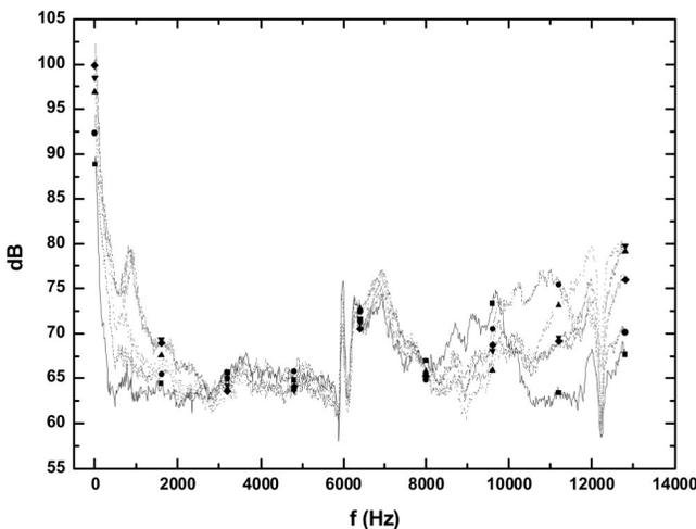
FIG. 10. Sound spectra measured at high flow rate in CO<sub>2</sub>. Divergent glottis-shaped orifice. ■,  $\Delta p = 10$  cm H<sub>2</sub>O; ●,  $\Delta p = 14$  cm H<sub>2</sub>O; ▲,  $\Delta p = 18$  cm H<sub>2</sub>O; ▼,  $\Delta p = 22$  cm H<sub>2</sub>O; ◆,  $\Delta p = 26$  cm H<sub>2</sub>O.
