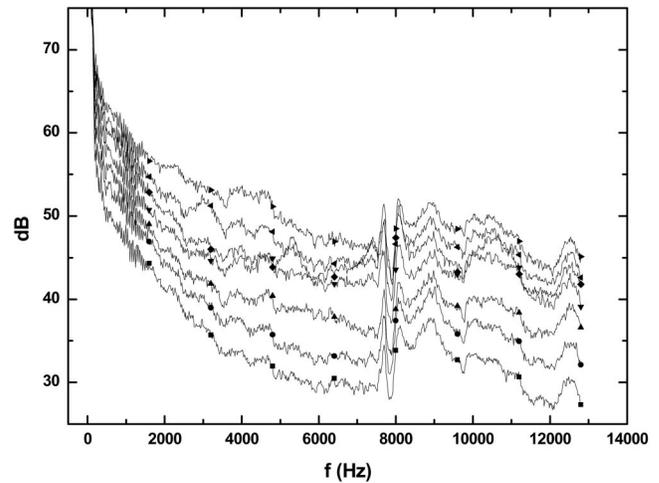
FIG. 4. Sound spectra measured for different transglottal pressure using air. Straight glottis-shaped orifice. ■,  $\Delta p = 8$  cm H<sub>2</sub>O; ●,  $\Delta p = 10$  cm H<sub>2</sub>O; ▲,  $\Delta p = 12$  cm H<sub>2</sub>O; ▼,  $\Delta p = 14$  cm H<sub>2</sub>O; ◆,  $\Delta p = 16$  cm H<sub>2</sub>O; ◀,  $\Delta p = 18$  cm H<sub>2</sub>O; ▶,  $\Delta p = 20$  cm H<sub>2</sub>O.
