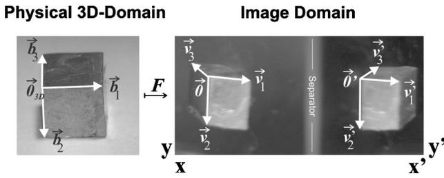
FIG. 3. Schematic representation of the LA method through means of the transformation matrix  $F$ . The left picture shows the brass cube in the physical domain, while the right picture shows the two camera views through the prism. Both camera views were assumed to preserve parallel projections.
