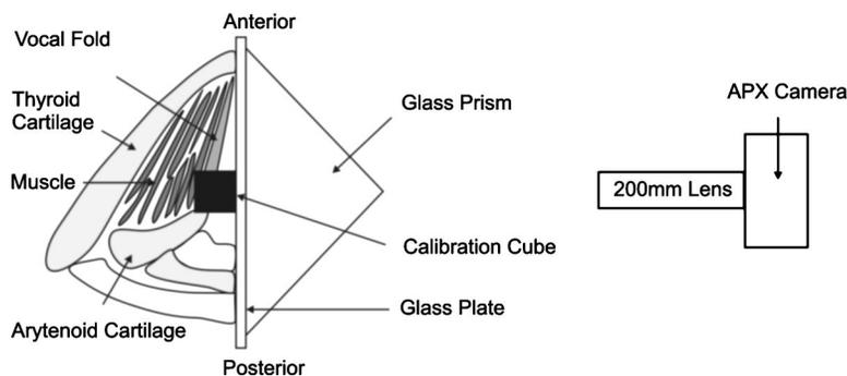
FIG. 1. A schematic representation of the experimental setup from a superior view: The glass plate, situated at the glottal midline, appears as a vertical line in the middle of the picture. The vocal fold and brass calibration cube are situated on the left side of the plate, and the glass prism and high-speed camera are situated on the right.
