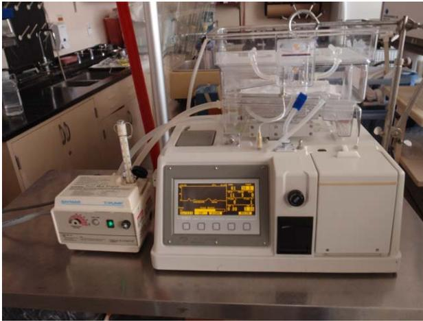
Fig. 2. RM3 pulsatile perfusion unit. The RM3 unit is displayed prior to priming with blood products. The circuit warmer is seen just to the left of the RM3, which maintains the perfusate at physiological temperatures. [Color figure can be viewed in the online issue, which is available at [www.laryngoscope.com](http://www.laryngoscope.com).]
