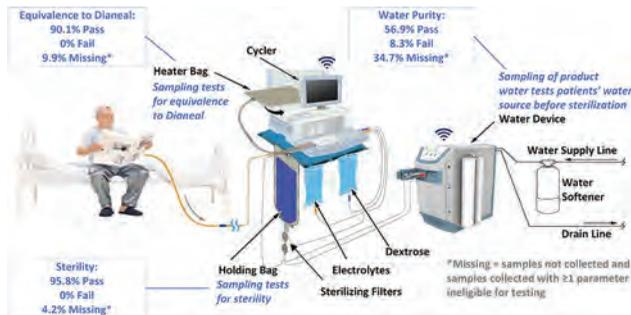
Figure 1. APD Solution Generation System and Main Results
