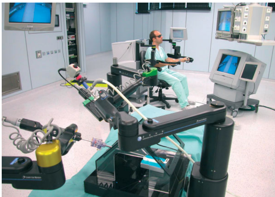
Fig. 1 Zeus™ robot set up for the knot-tying test. Effector arms are shown in the foreground with surgeon and actuator controls in the background
