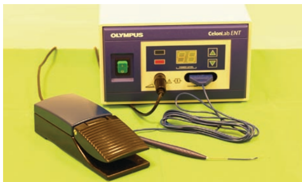
Fig. 7.1.1 Radiofrequency generator Celon with foot switch
