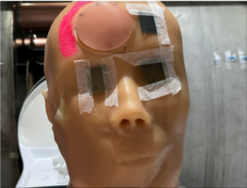
Figure 1: Films placed inside the insert, on the forehead and on the lens to evaluate dose.
