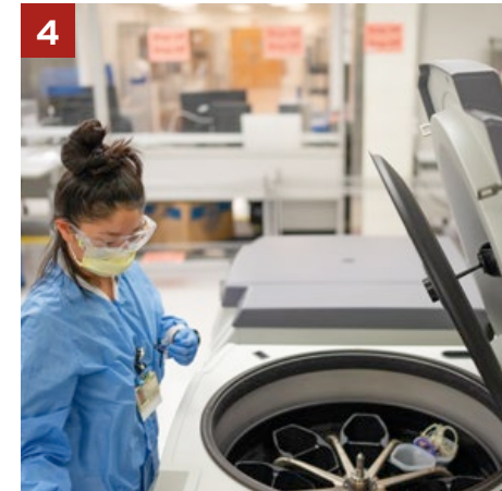
4 The donated blood is placed into a centrifuge to separate the red blood cells and plasma. Photo: Milo Mitchell/UCLA Health
